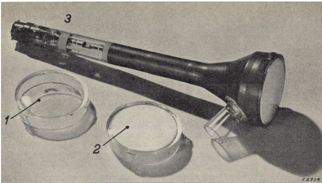
Fig. 2. 1 = tube face before the luminescent screen has been applied, 2 = tube face with luminescent screen, 3 = the complete tube MW 6-2.
