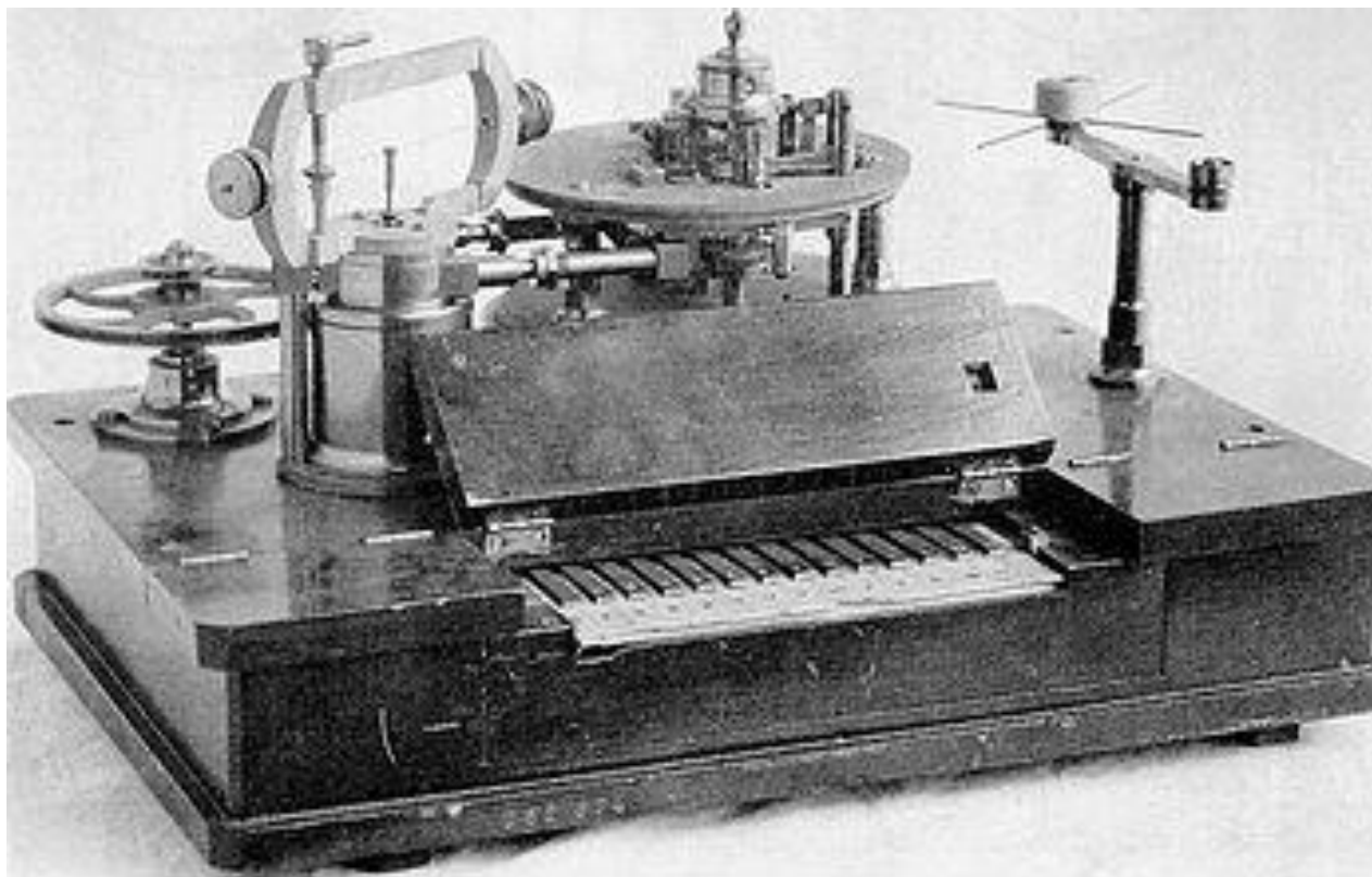
(Photograph courtesy of Smithsonian Institution, Washington, D.C.) 1845 PATENT OFFICE MODEL OF HOUSE'S PRINTING TELEGRAPH
