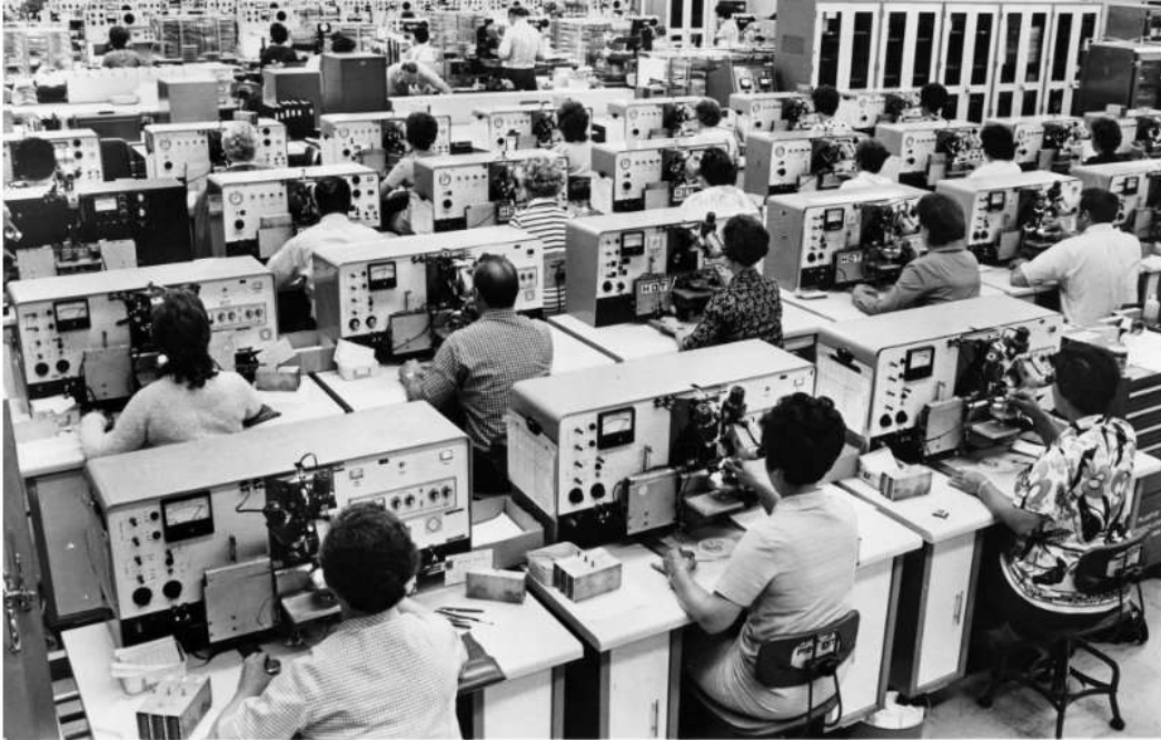
CURRENT PRODUCTION of diffused silicon plastic-encapsulated transistors at Western Electric's Allentown Works shows progress that has been made in 25 years by mechanization of production of discrete transistors. During the chip and lead-bond operations, transistor chips are handled by vacuum pick-up needles and connected by 0.001 inch diameter gold wire fed through a hollow point needle. These assembly steps are controlled by operators peering through microscopes. Testing is done largely by computer-controlled test systems. WE transistors are used in major carrier and electronic switching systems and other Bell System applications. TA-2
